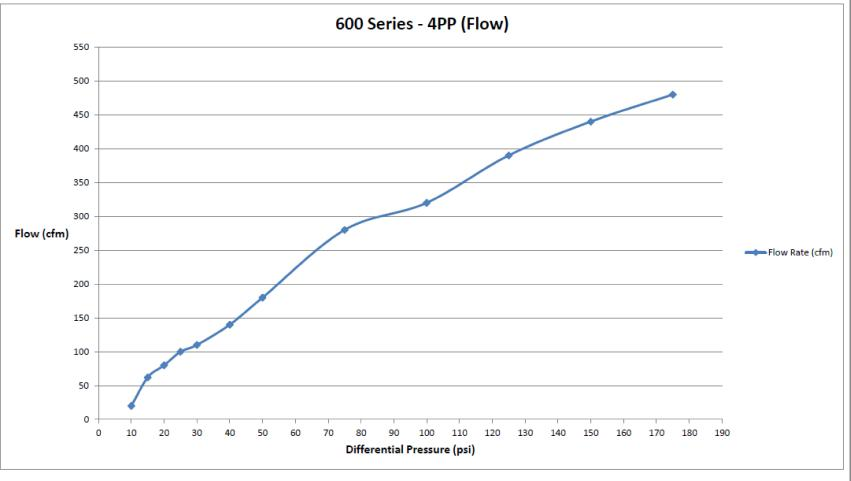
**Differential Pressure** is define as the change in pressure between the inlet pressure minus the crack pressure
