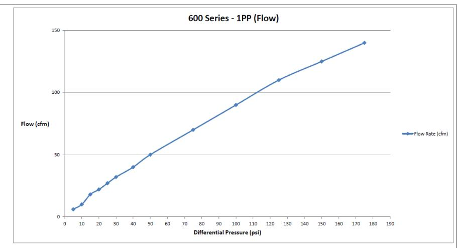
**Differential Pressure** is define as the change in pressure between the inlet pressure minus the crack pressure
