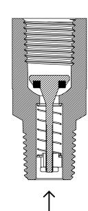
Body Material: Aluminum\*, Brass\*, 303 SST\*, 316 SST\*, 17-4 SST, 12L14
