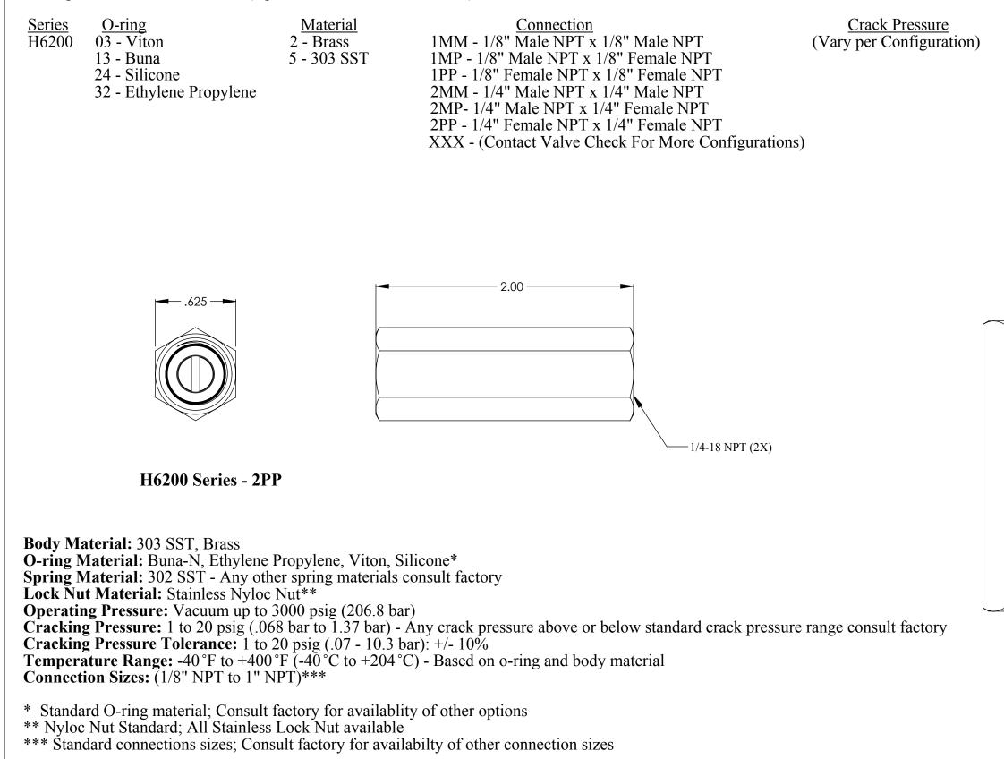
Note: 1. Proper filtration is recommended to prevent damage to the o-ring or sealing surface
